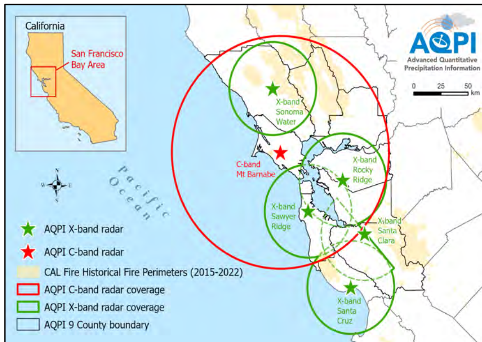
Figure 1: Schematic of AQPI radar deployments across the Greater San Francisco Bay Area. The green stars and circles represent X-band radar locations and coverage areas. The red star and circle represent C-band radar location and coverage area. Gray lines represent county boundaries and tan shading indicates historical fire perimeters from 2015–2022. Note that the X-band in Santa Cruz, while closely integrated with AQPI, was procured separately and is not part of this financial agreement.
