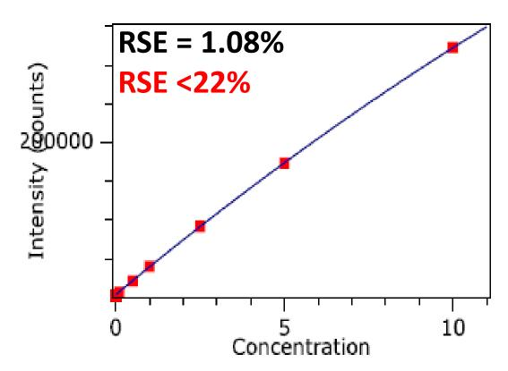
MDL = 0.02 mg/L RL = 0.1 mg/L
