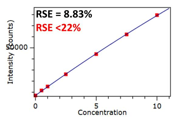
MDL = 0.16 mg/L RL = 0.5 mg/L
