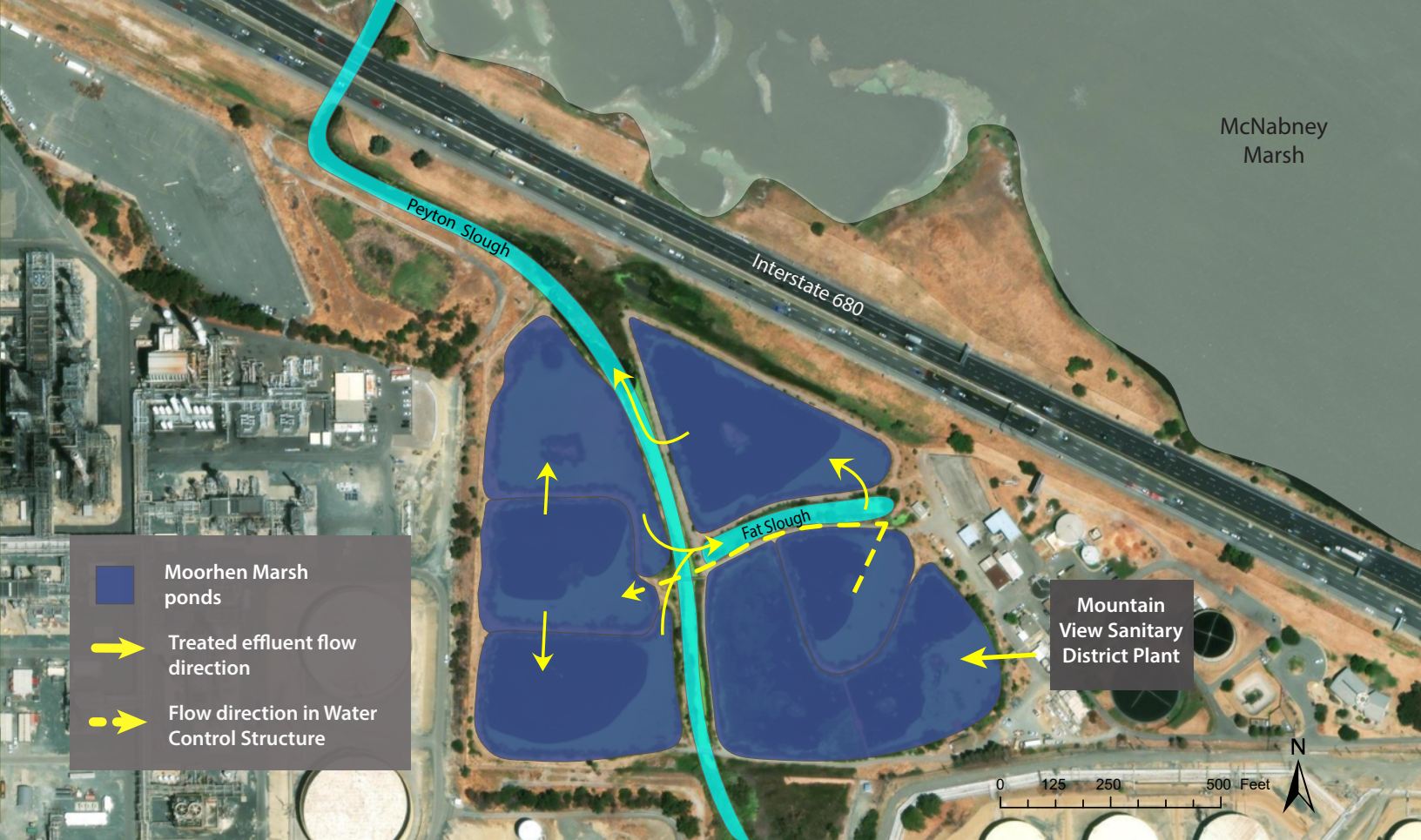
Diagram of Moorhen Marsh. The 20-acre constructed wetland is made up of six ponds and a connecting slough to McNabney Marsh.
