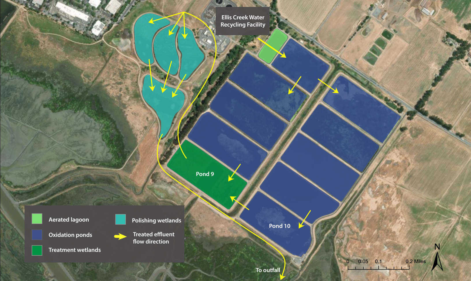
Diagram of the Ellis Creek wetlands. The site includes an aerated lagoon, oxidation ponds, treatment wetlands, and a 31-acre polishing wetland, with effluent discharged into the Petaluma River.
