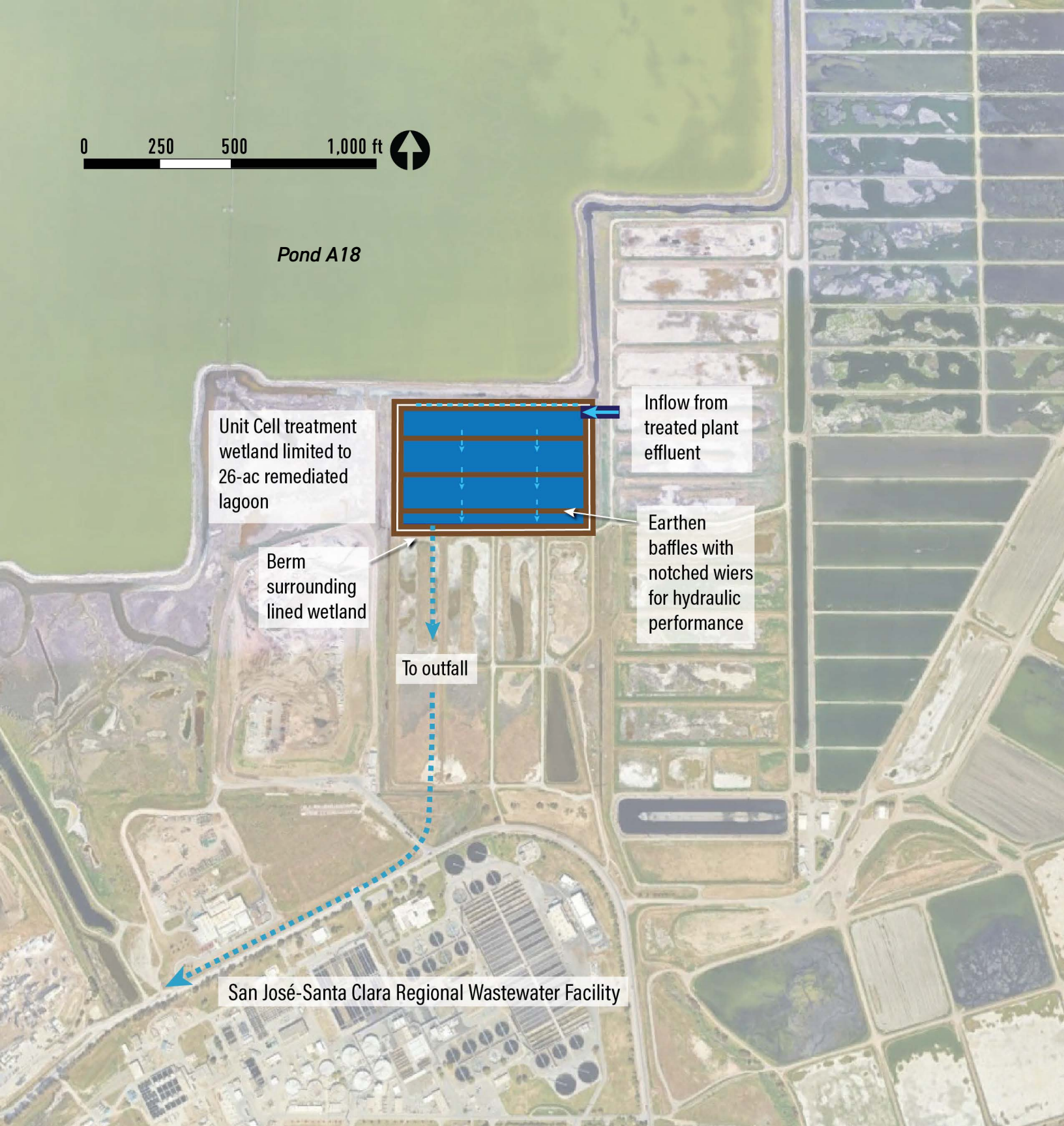
Figure 1. Option 1, encompassing 26 acres of open water treatment wetlands on the remediated lagoons resulting from Phase 1 of the Cleanup Project.
