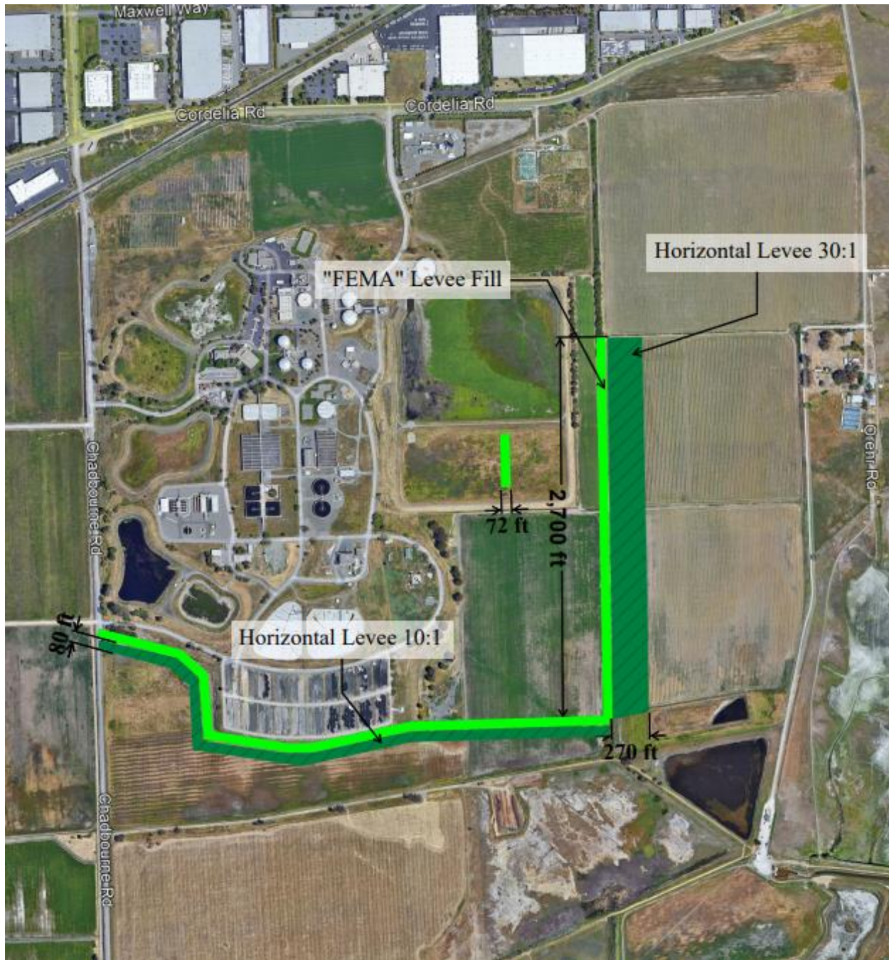
Figure 2. FSSD: Horizontal Levee with a 30:1 Slope Horizontal Levee on the East side and a 10:1 Slope on the South
