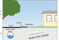
This program only applies to a sanitary sewer line lateral, which is the pipeline that carries wastewater from the building to the property line. Property owners are responsible for all costs relating to
