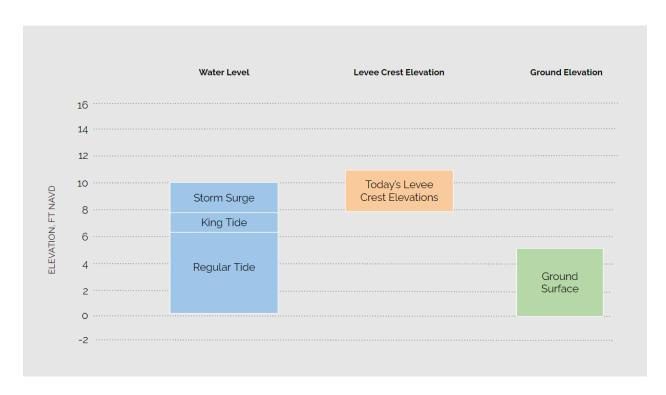
**Figure 5.** Ranges of water surface elevations, ground surface elevations of diked baylands, and levee crest elevations in the diked baylands on the eastern side of the Petaluma River. Elevation data from Buffington and Thorne (2019).
