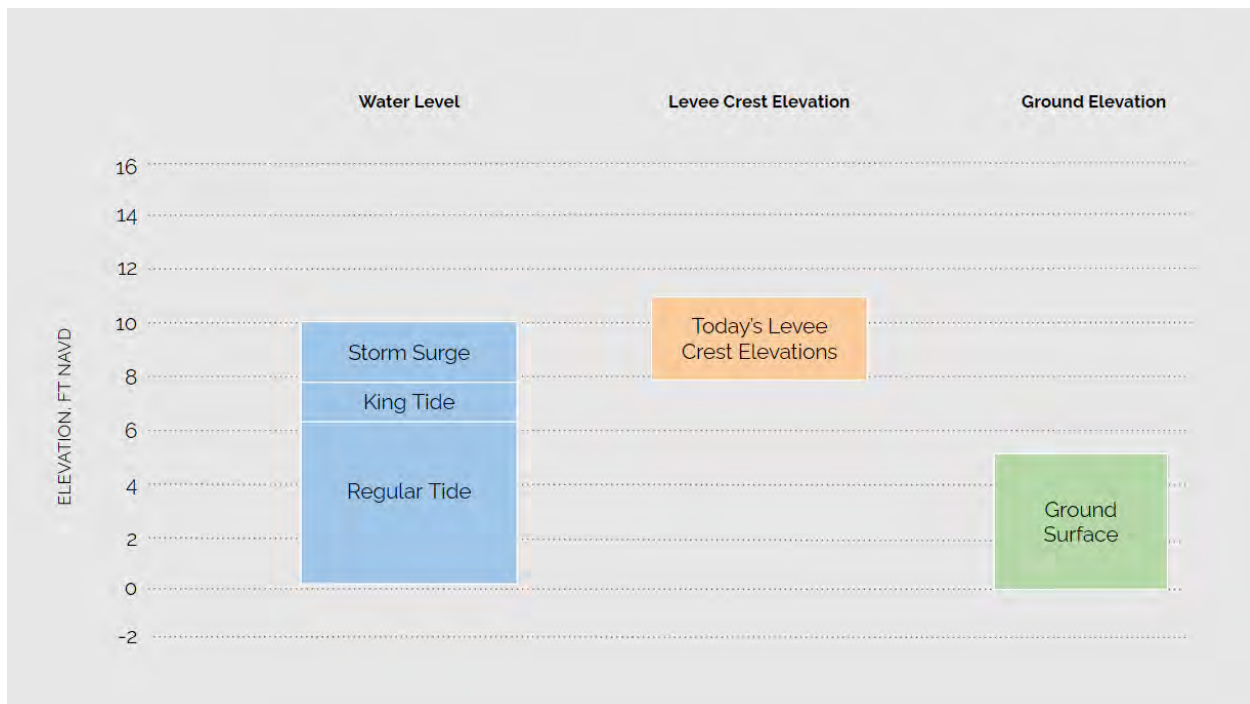
Figure 5. Ranges of water surface elevations, ground surface elevations of diked baylands, and levee crest elevations in the diked baylands of the eastern side of the Petaluma River. Elevation data from Buffington and Thorne (2019).
