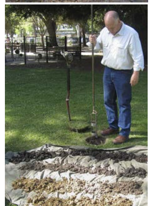
Soil profiles are investigated by digging backhoe pits (top) or using a bucket auger (bottom) to remove soil to four feet deep or more. Soils that comprise the profile are described and samples collected at appropriate depths.
