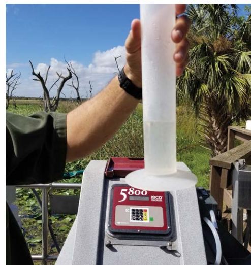
In-field water quality monitoring of reclaimed water is conducted at a Florida water reuse facility to ensure fit-for-purpose specifications are being met.
