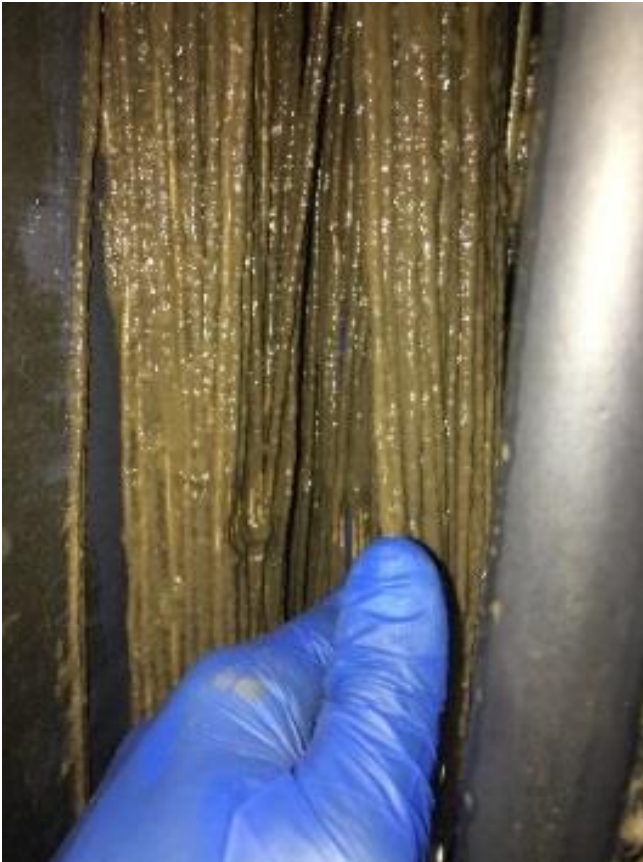
HIGHER LOADING CONDITIONS (Sol. COD Loading \sim 40 \text{ g/m}^2\cdot\text{d} )
