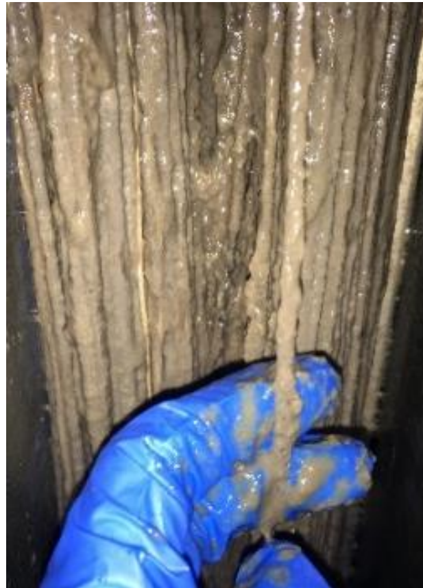
HIGHER LOADING CONDITIONS (Sol. COD Loading \sim 40 \text{ g/m}^2\cdot\text{d} )
