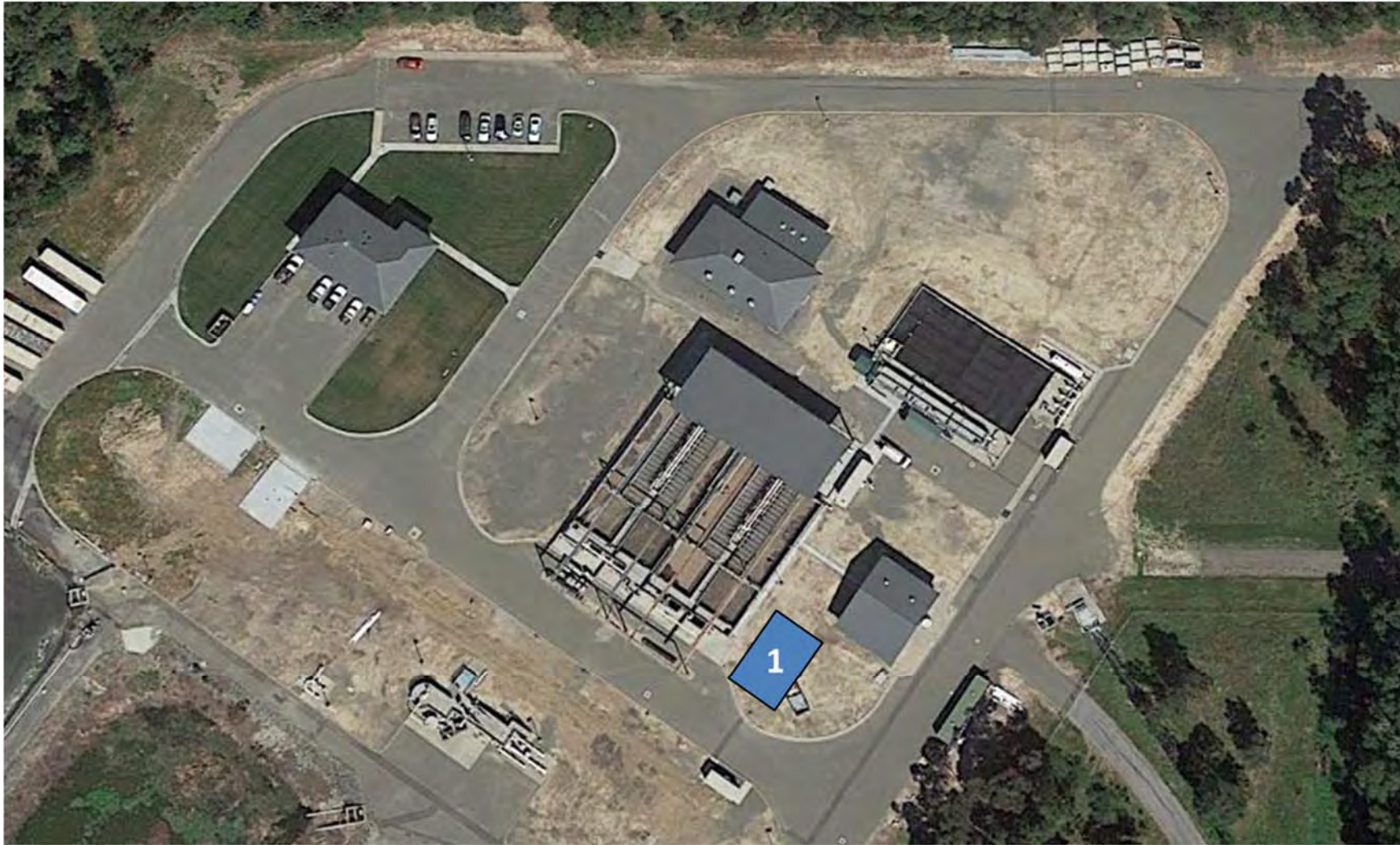
Figure 6-3. Level 2 Upgrade Aerial Layouts for Dry Season and Year Round (1) construct facilities for alum addition
