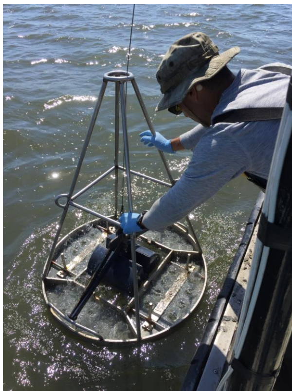
Figure 3.1 Deploying a Van Veen grab for sediment sample collection.
