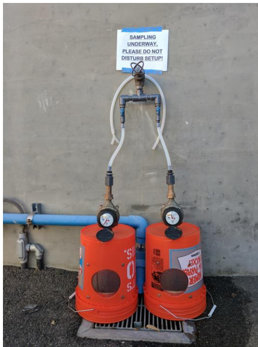
Figure 3.3 Wastewater effluent sample collection setup. Microplastic wastewater effluent samples were collected by connecting a flowmeter to the effluent sampling valve, and collecting particulates from effluent flow in two sieves that were placed under an upside down bucket. Duplicate samples were collected at one wastewater treatment facility. Sampling train designed by City of Palo employees.
