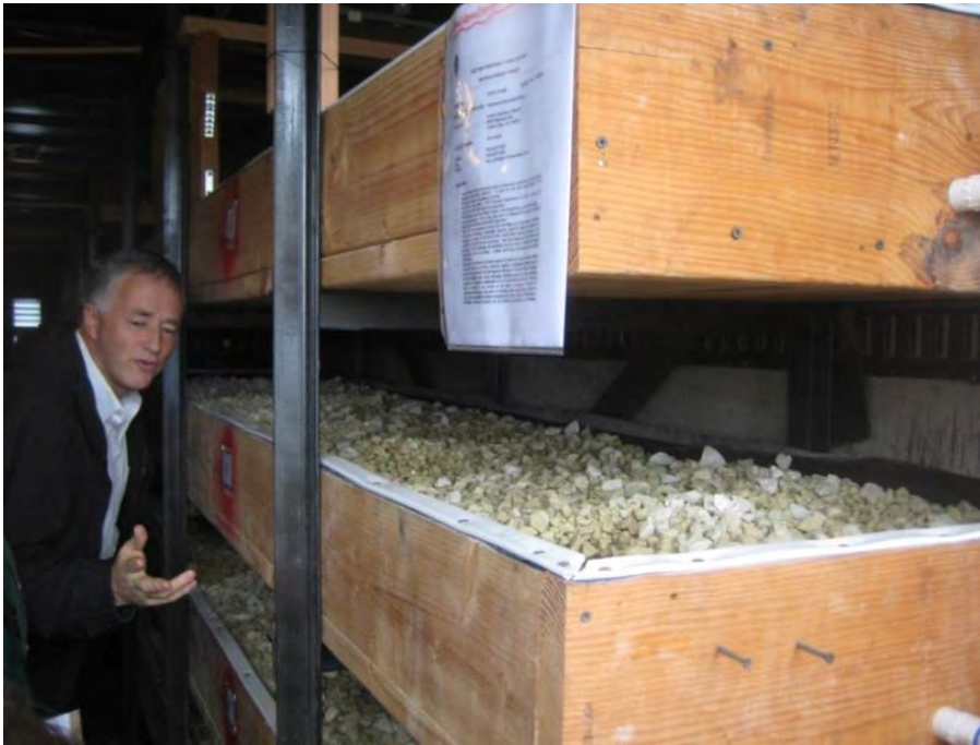
Figure 28. Zeolite/anammox Pilot Beds at Union Sanitary District in 2012.
