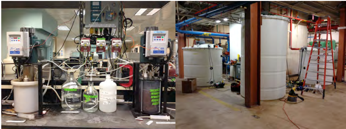
CANDO systems at Delta Diablo: bench-scale (left), pilot-scale (right).
