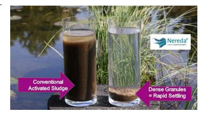
Use of a sequencing batch approach negates the need for a secondary clarifier, further saving space and conserving energy. Nereda® has reportedly been shown to use approximately 30-40% less energy than conventional flow-through CAS, in part due to the absence of recycle pumping for Internal Mixed Liquor Recycle (IMLR) and Return Activated Sludge (RAS).
