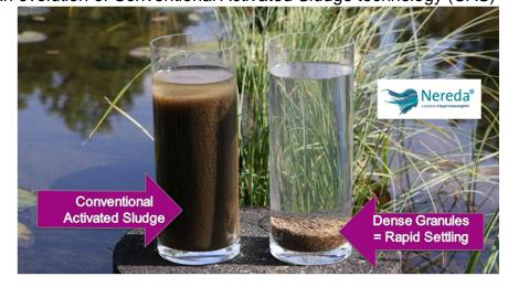
enforcing strict feast-famine feeding regimes in Sequencing Batch Reactors (SBRs) ensuring selection of phosphate-accumulating organisms (PAOs), thereby removing phosphorus as
