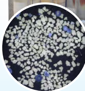
Optical microscope photo of microbeads extracted from off-the-shelf personal care products showing rounded, bead-like pellets along with more plentiful, rough plastic fragments. Courtesy Sherri A. Mason.
