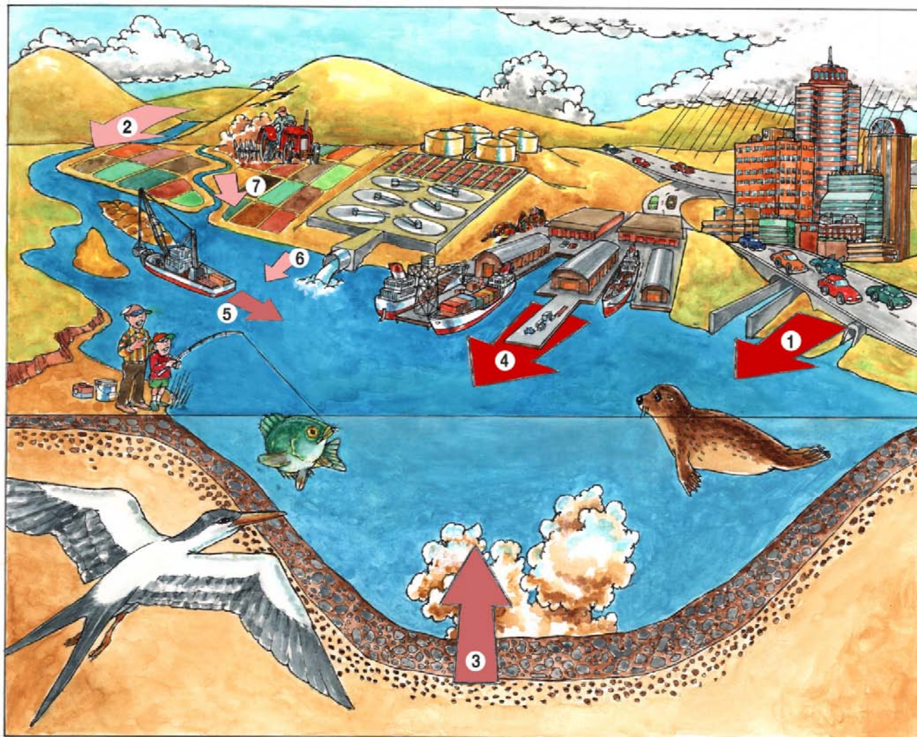
Figure 9. PCB pathways to the Bay: 1) urban runoff; 2) Central Valley (Delta outflow); 3) buried sediment; 4) in-Bay PCB hot spots; 5) dredging and dredged material disposal; 6) wastewater effluent; and 7) nonurban runoff. Not shown: atmospheric exchange. The size of each arrow indicates the relative magnitude of the load. The color of each arrow indicates how concentrated the input stream is (darker colors more concentrated). Urban runoff, the Central Valley, erosion of buried sediment, and in-Bay hot spots likely represent the largest pathways.
