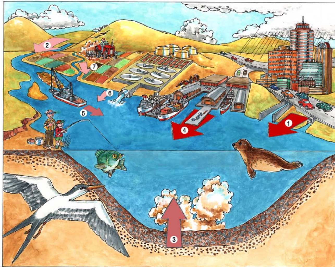
Figure ES-4. PCB pathways to the Bay: 1) urban runoff; 2) Central Valley (Delta outflow); 3) buried sediment; 4) in-Bay PCB hot spots; 5) dredging and dredged material disposal; 6) wastewater effluent; and 7) nonurban runoff. Not shown: atmospheric exchange. The size of each arrow indicates the relative magnitude of the load. The color of each arrow indicates how concentrated the input stream is (darker colors more concentrated). Urban runoff, the Central Valley, erosion of buried sediment, and in-Bay hot spots likely represent the largest pathways.
