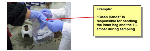
3. "Clean Hands" holds the sample container during collection. "Clean Hands" must be very careful to assure the 1 L amber does not touch any surfaces to prevent contamination and to hold the cap down in the other hand.
