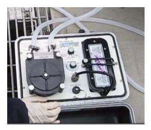
6. Fill the desired number of sample bottles via the discharge tubing being careful not to remove the inlet tubing from the water.
