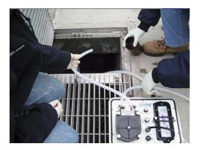
d. Dedicated Sampling Port Procedure-This is a sampling procedure where no pumping equipment is used. A dedicated sampling point with a representative continuous flow is used to sample for Dioxin/Furans.
