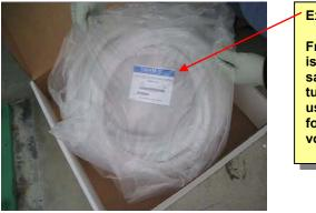
Example: Fresh silicon tubing is used for each sampling event. Used tubing can be reused after cleaning for other semivolatile sampling.
