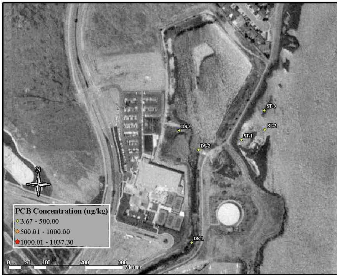
Figure 4. Coring Locations and Relative PCB Concentrations ( \mu\text{g}/\text{kg} ) at Steinberger Slough / Delta Star Site.
