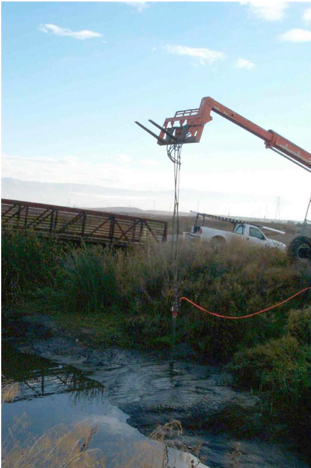
Figure 3. Coring Equipment Being Deployed via Forklift at East Sunnyvale Creek
