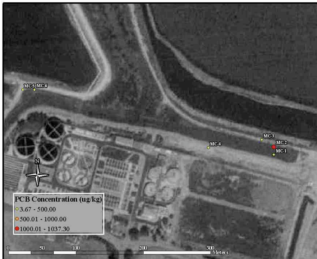
Figure 9. Coring Locations and Relative PCB Concentrations ( \mu\text{g}/\text{kg} ) at Moffett Channel Site
