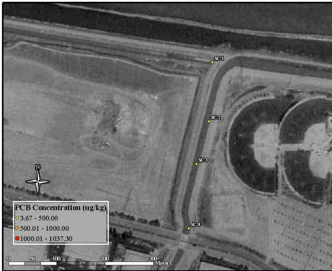
Figure 8. Coring Locations and Relative PCB Concentrations ( \mu\text{g}/\text{kg} ) at East Sunnyvale Creek Site
