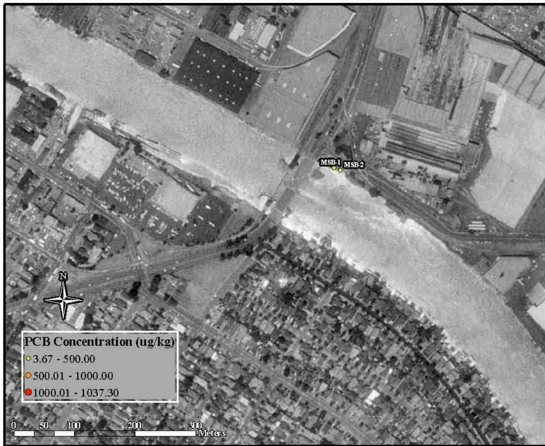
Figure 5. Coring Locations and Relative PCB Concentrations ( \mu\text{g}/\text{kg} ) at Miller Sweeney Bridge Site. Core location markers were adjusted manually to better represent actual coring locations relative to channel.
