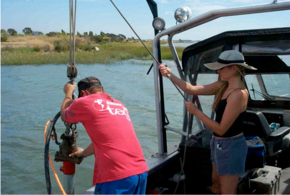
Figure 2. Coring Equipment Being Deployed from a Shallow Draft Vessel within San Leandro Bay
