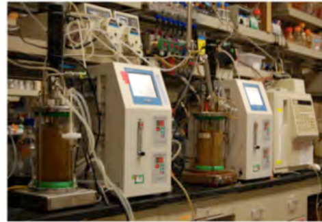
Bench-scale testing of CANDO with real wastewater
