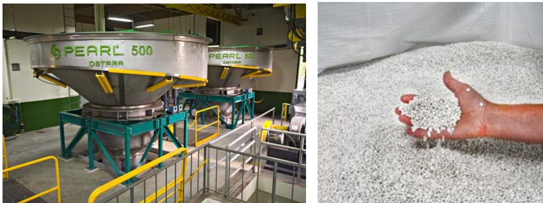
Figure 8. Image of a MAP Reactor from Ostara® (Left) and the MAP Crystal from Ostara® (Right)
