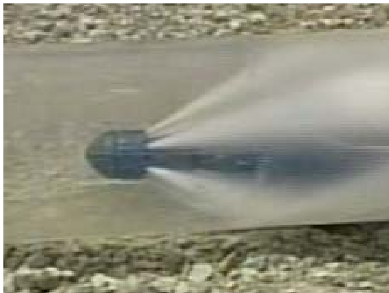
Figure 3-1, Nozzle in Clear Pipe
