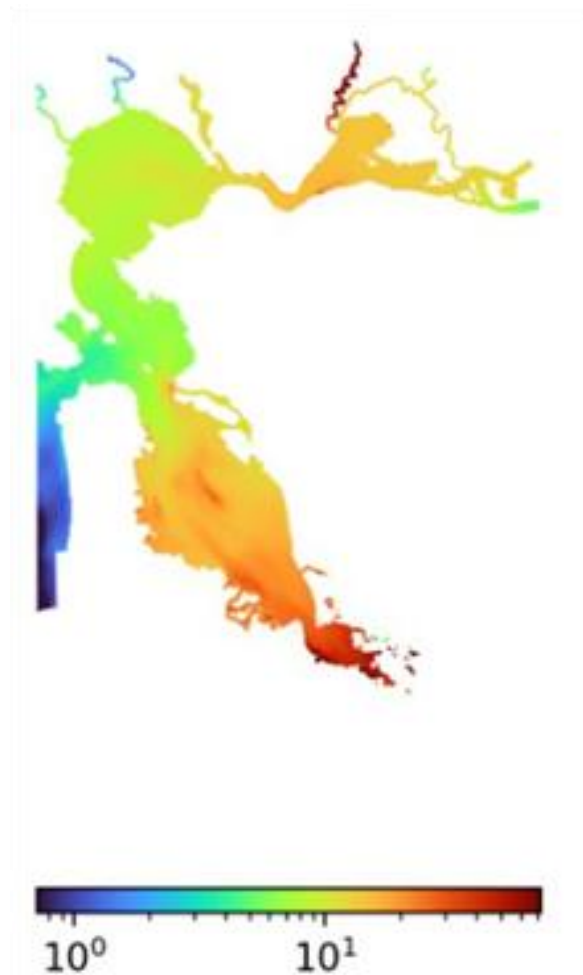
Figure 2. Example of SFEI's TIN Source Apportionment Model, showing concentrations of tracer (representing Dissolved Inorganic Nitrogen) in micromolar. 18
