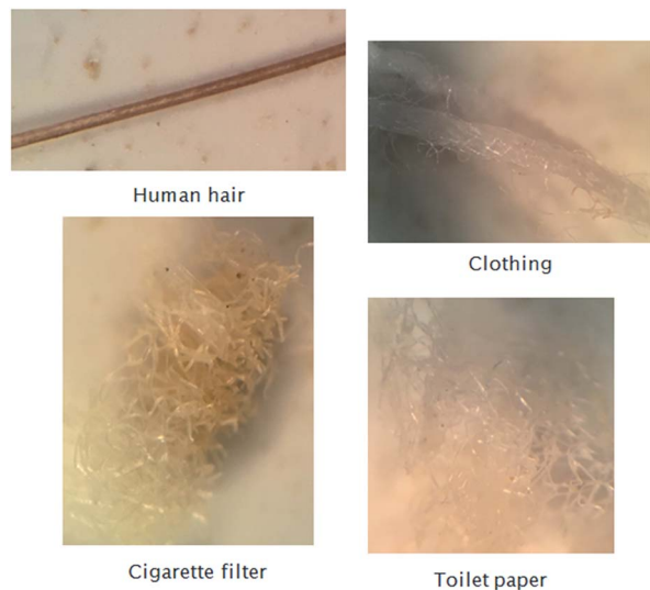
Fig. 6 Non-microplastics after WPO digestion.
